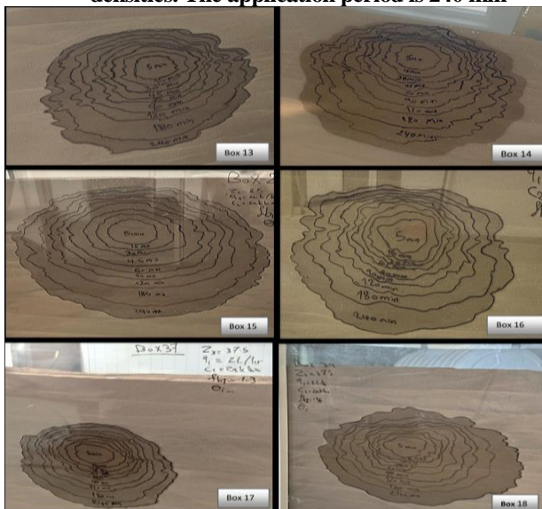
Figure 7: Six experimental boxes (13-18) labeled for Zakho soil, which were designed to test the effects of three emitter installation depths and two different discharge rates for different soil bulk densities. The application period is 240 min
