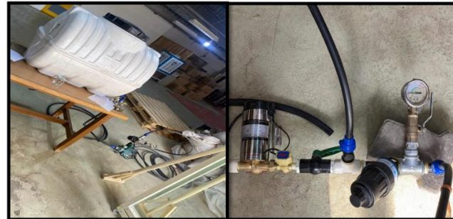
Figure 4: Pump–pressure gauge assembly used to provide controlled water pressure for soil box irrigation
