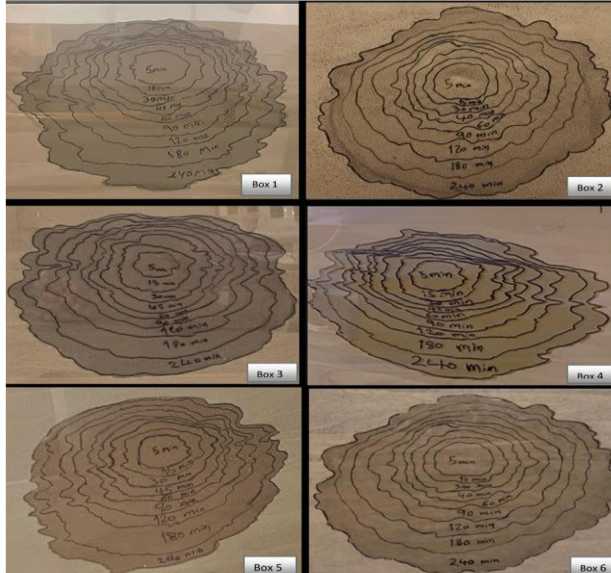
Figure 5: Six experimental boxes (1-6) labeled for Semel soil, which were designed to test the effects of three emitter installation depths and two different discharge rates for different soil bulk densities. The application period is 240 min
