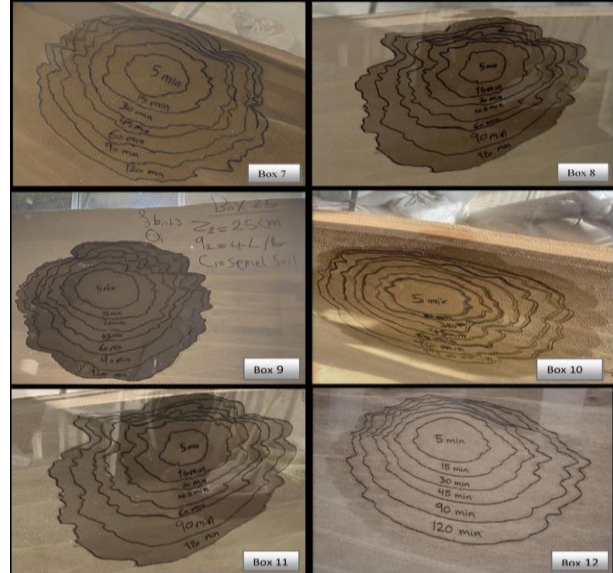
Figure 6: Six experimental boxes (7-12) for Semel soil, designed to assess the effects of three emitter installation depths and two different discharge rates under different soil bulk densities. 120 min application water
